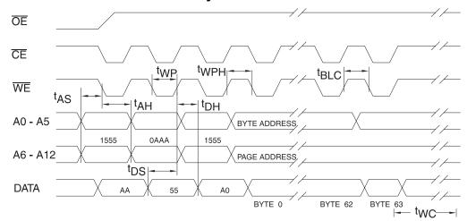
Notes: 1. A0 - A12 must conform to the addressing sequence for the first three bytes as shown above.
